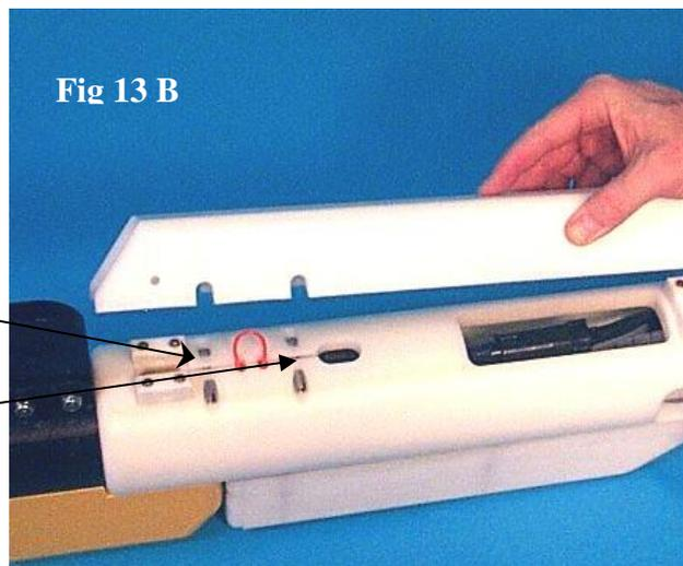
Loosen these screws to also rotate the nose. **Do not remove the orange locking strings.**
