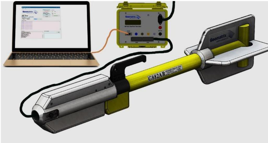
**Figure 42** Typical test setup G-882 digital powered by a Geomatrix GP102 Tow Fish Test Box (in D9 mode) with a Laptop running G-882 digital Console
